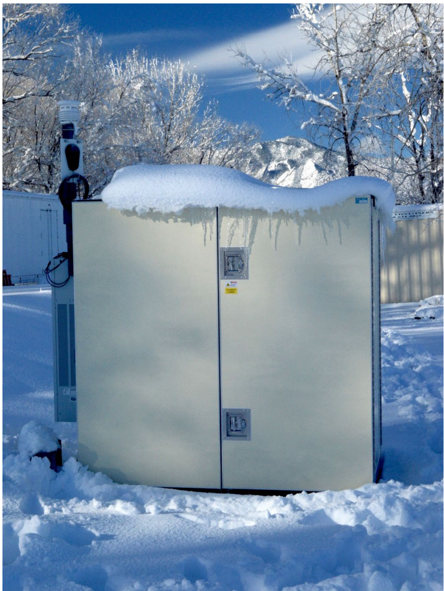
Water Vapor DIAL profiling system, courtesy of NCAR
