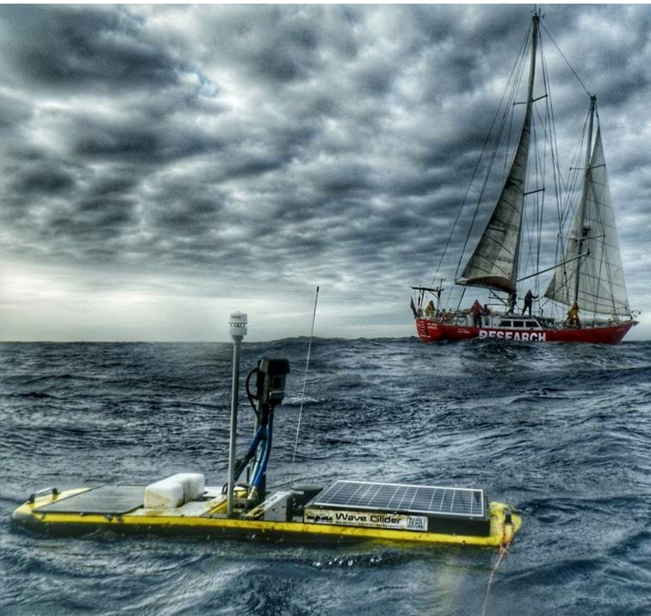
Wave Glider with carbon system, from CSIR
