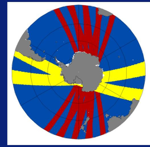
Locations of ground swaths during a "typical" 3-hour period (3-6am GMT) for ASCAT-2 and ASCAT-3 (red) and Zephyr (yellow). Note the separation in space that provides the "6-hour separation in time.
