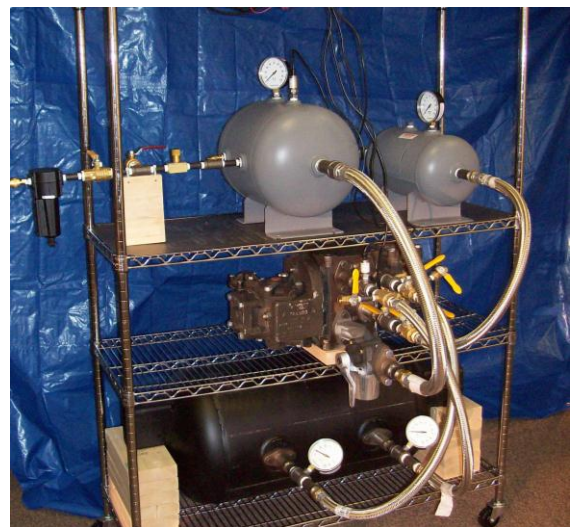
Figure 11. Single-car brake system test fixture for control valve characterization
