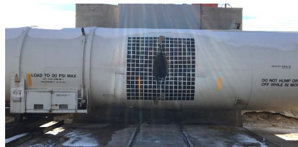
Figure 2. Post-test Photo of the Punctured Shell
