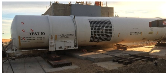
Figure 1. Pre-test Photo of DOT-113 Tank Car
