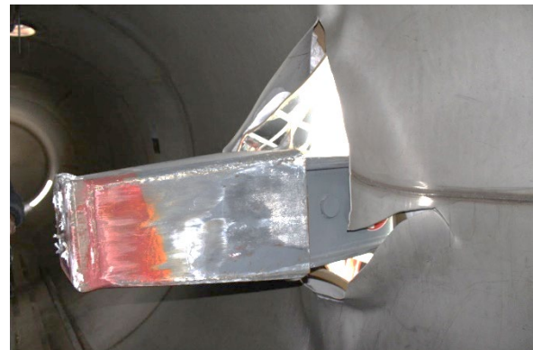
Figure 6. Post-test Tear in Inner Tank
