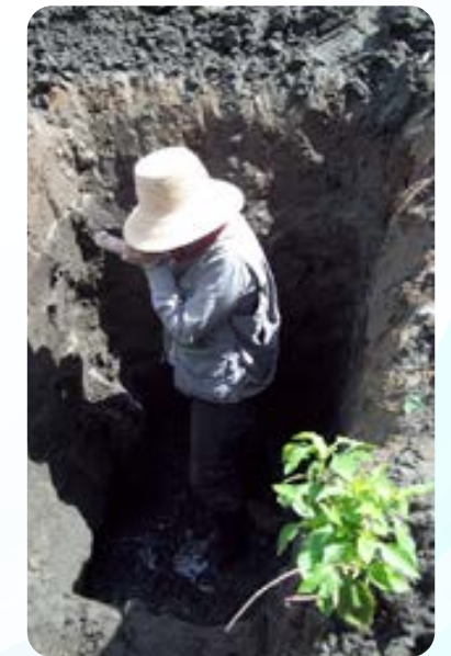
Sampling floodplain sediment using a trench of 170 cm depth, Colombia
