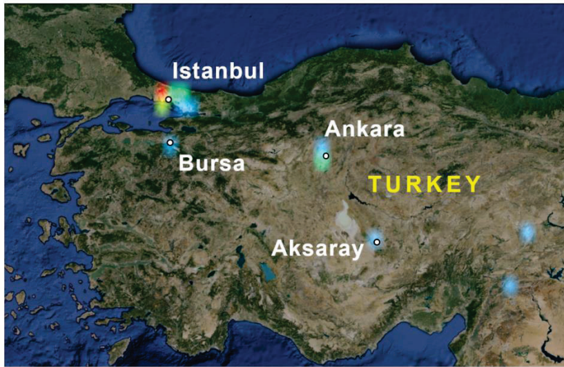
FIGURE 1: Example of emissions within the 23.6-24.0 GHz band consistent with radio frequency interference contamination in Turkey. Counts of AMSR2 23.8 GHz (vertically polarized channel) radiances >310 K during 2022, indicating low emission levels in blue, medium levels in green, and high levels in red. SOURCE: Committee generated
