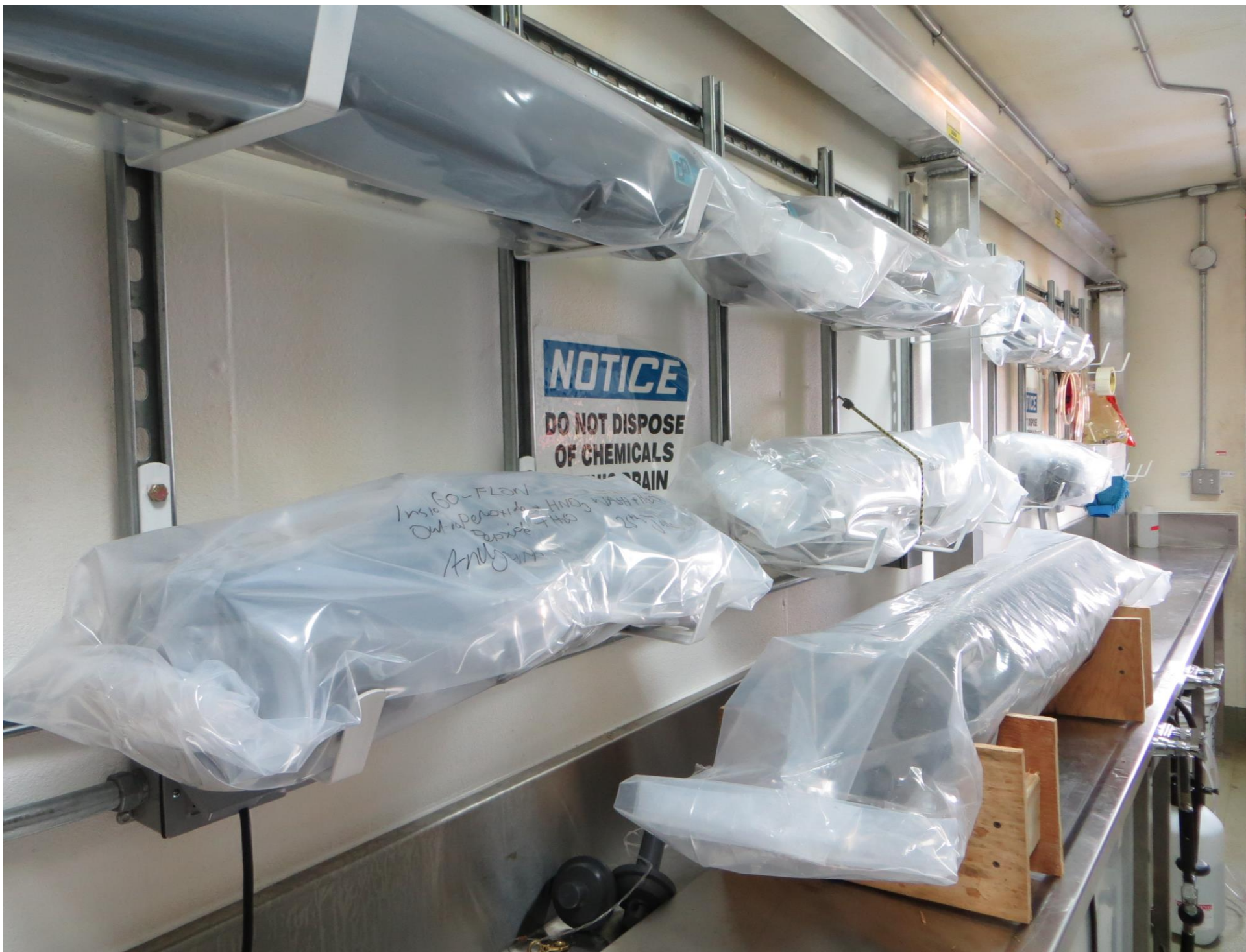
Instruments in bags after cleaning with H 2 O 2
