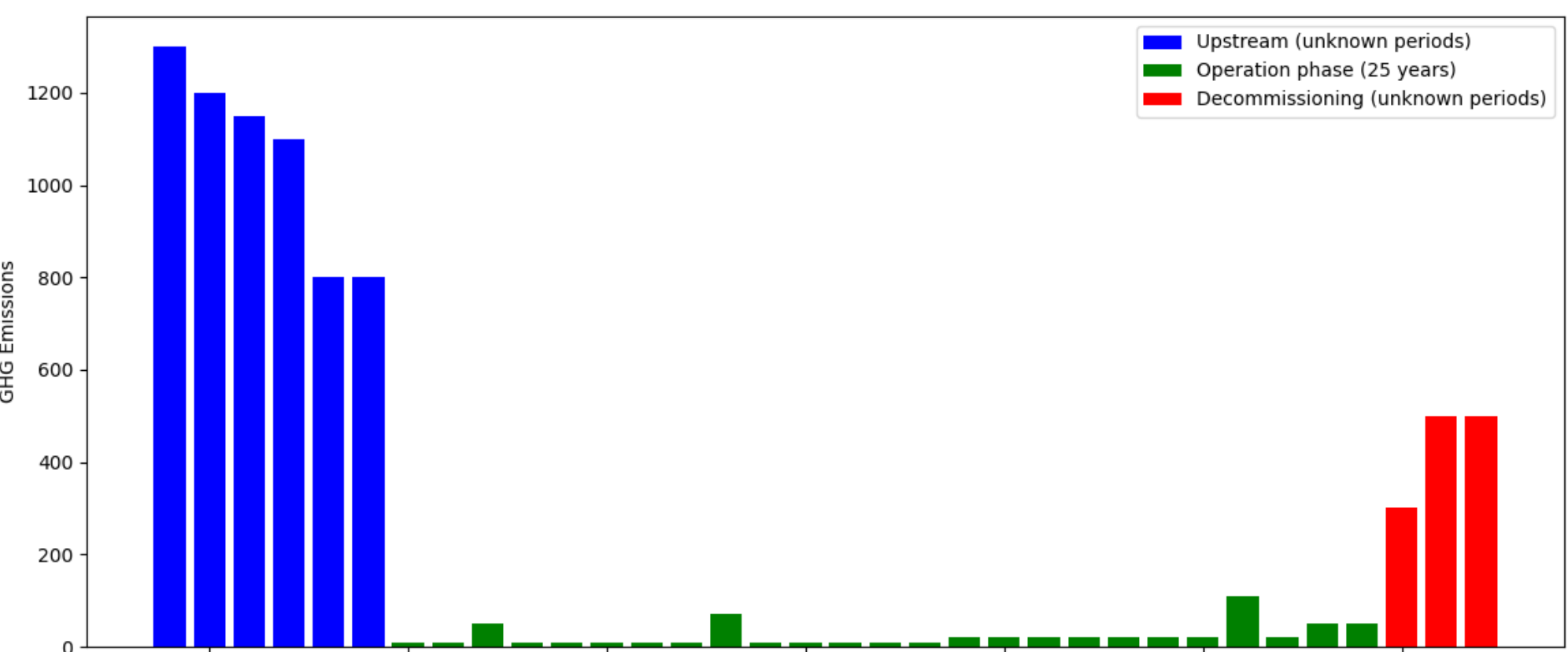
Figure 2: Conceptual graph of the timing of GHG emissions along the life cycle of a renewable electricity generation system.
