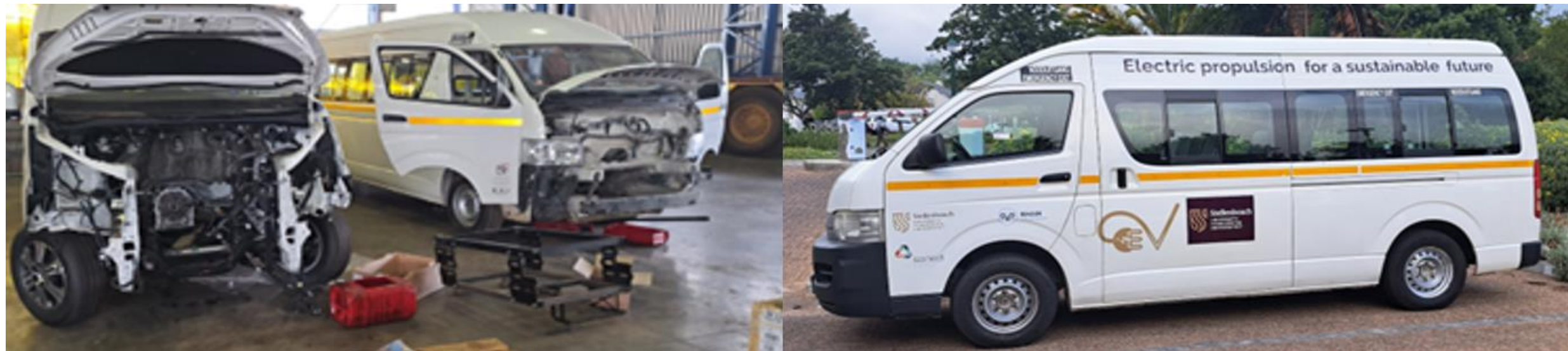
Figure 3. Retrofitting internal combustion engine vehicles to electric propulsion in South Africa
