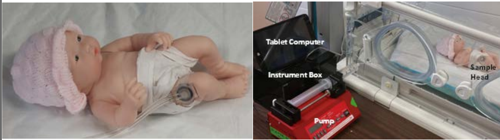
Figure 1 Noninvasive glucose monitoring system for the neonatal intensive care unit: (left) Sample head for the noninvasive transdermal measurement of glucose on the thigh of the neonate; (right) the complete system showing the instrumentation.
