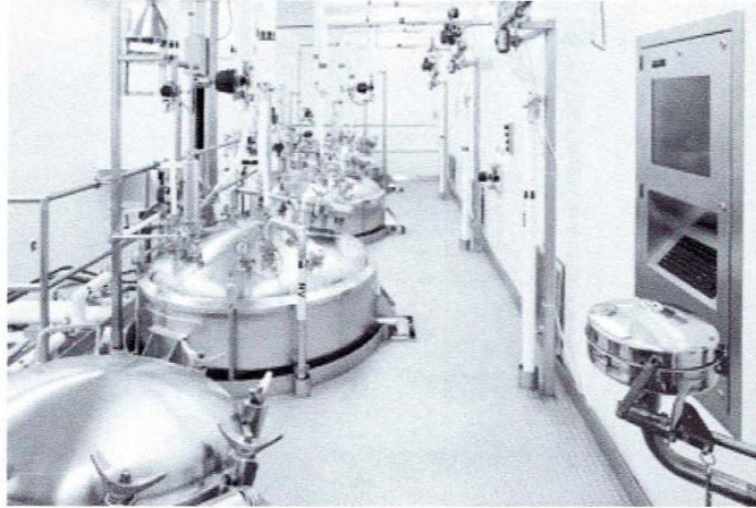
Tanks for tangential flow diafiltration
