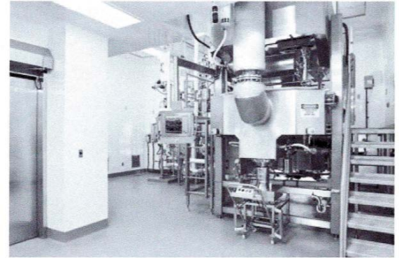
Cryogranulator used to form Technosphere Insulin pellets prior to lyophilization
