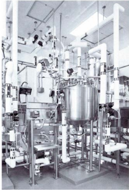
Tanks for tangential flow diafiltration
