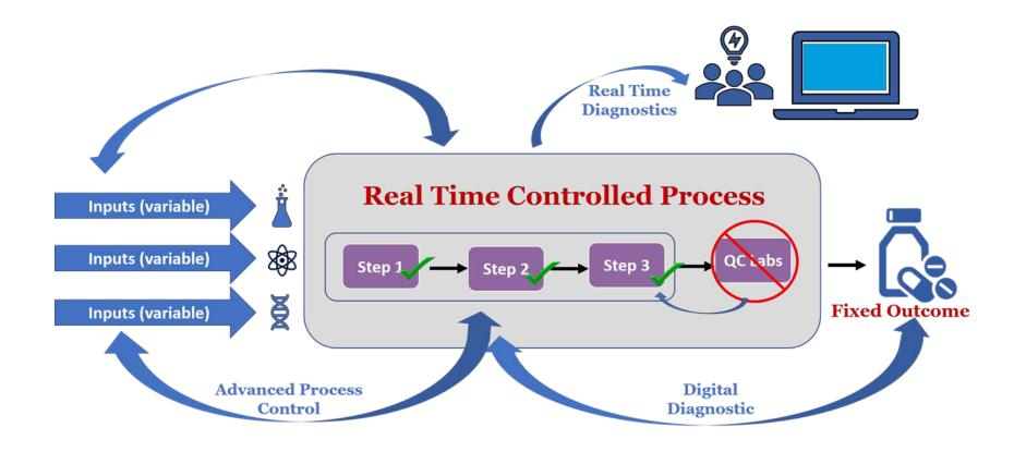
This represents a fundamental shift for ensuring process control and reliability. Move from sample and test to real time awareness
