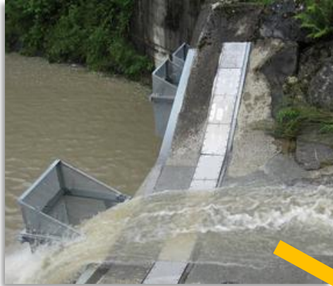
Sediment transport rates independently constrained by in-bed geophone system
