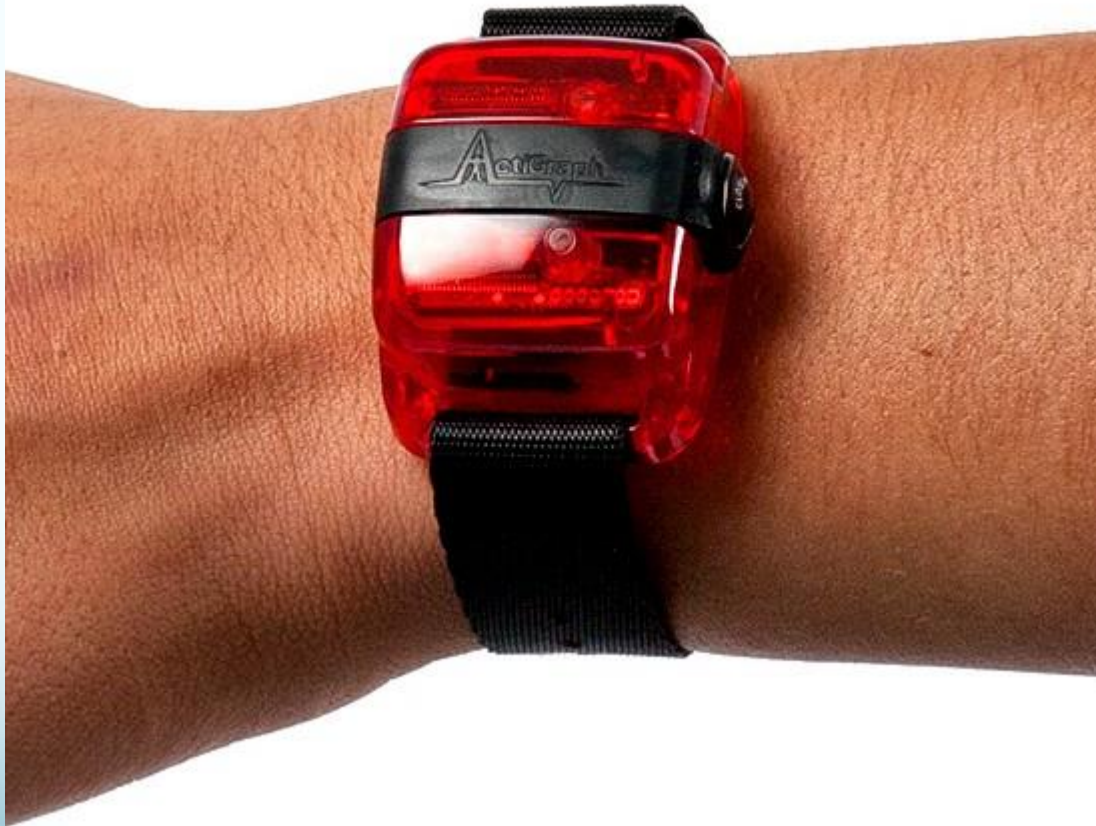
ActiGraph wGT3X-BT for accelerometry
