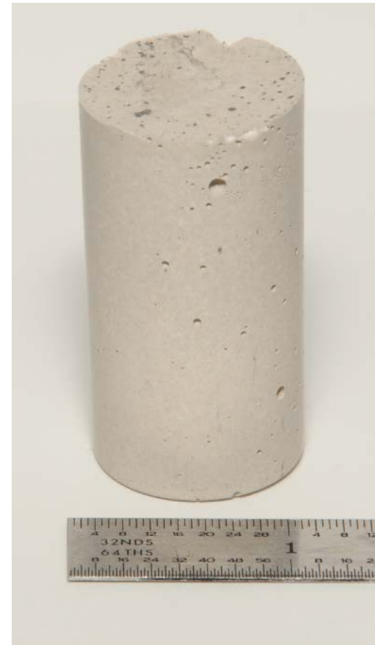
(b) 1173 Bed product (sectioned) from 2004 Pilot Scale Testing
