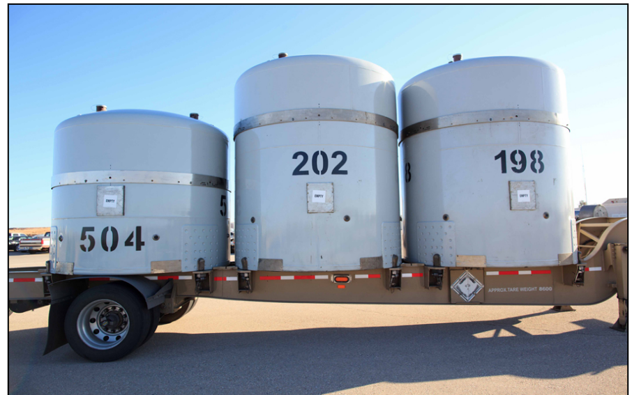
Type B Cask HalfPACT cask (left side of trailer) Contact-handled, 30 watts max Weigh ~ 10,500 lb & carry 7,000 lb
