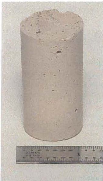
Figure 4-2. Troy clay geopolymer monolith of Hanford LAW 60% FBSR product (SRNL-ORNL-PNNL-WRPS downselect 2015).
