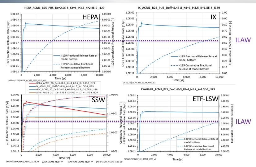
Modeled assuming oxidized conditions for a typical Hanford waste grout (no getters) in the waste forms.
