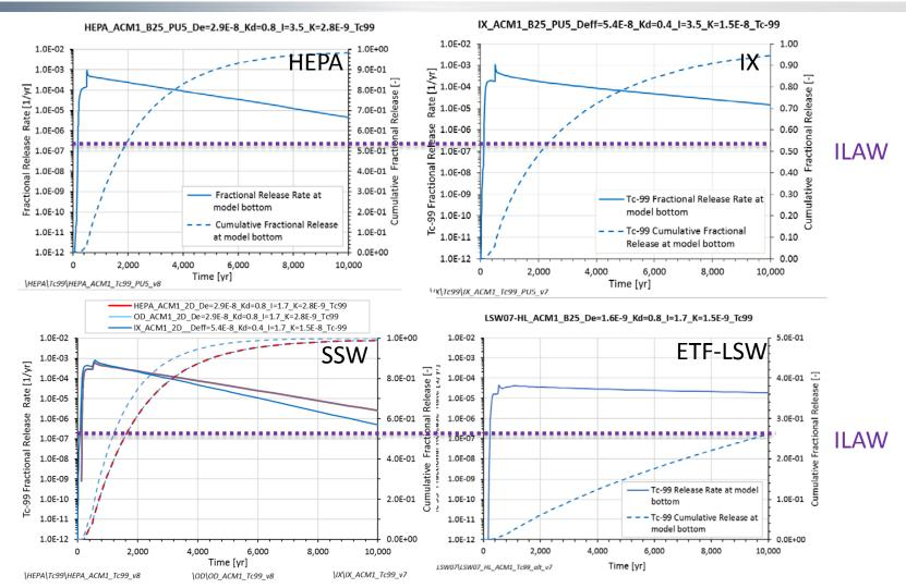
Modeled assuming oxidized conditions for a typical Hanford waste grout (no getters) in the waste forms (increased mobility of Tc-99).
