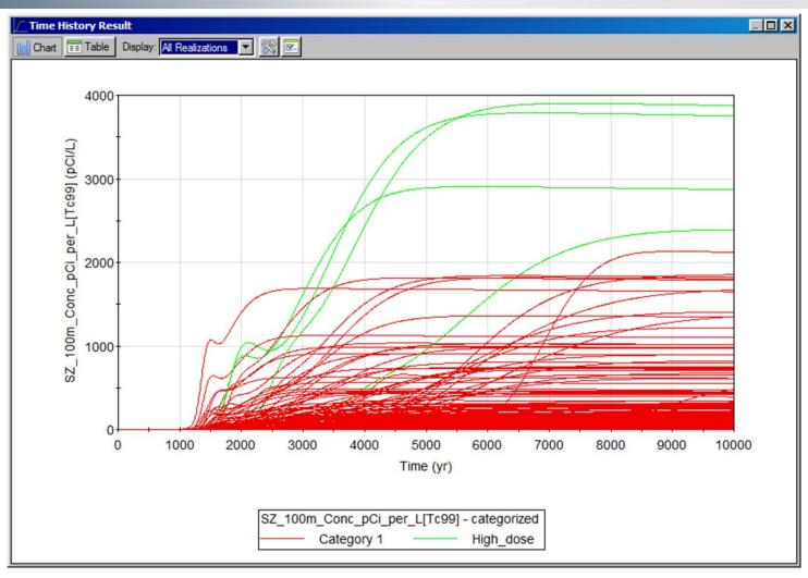
Mean = 0.035 pCi/L @ 1,000 years and 250 pCi/L at 10,000 years. Median = 0.0 pCi/L @ 1,000 years and 77 pCi/L at 10,000 years.
