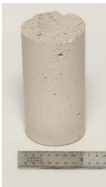
Figure C-14 Troy clay geopolymer monolith of Hanford LAW 60% FBSR product (SRNL-ORNL-PNNL-WRPS downselect [Jantzen 2015a]).
