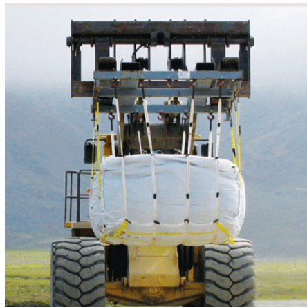
Figure H-7. Example of Soft Side Container for Shipping LSA Materials (photograph from PacTec, Inc literature 106 )
