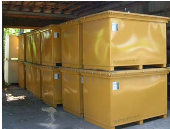
Figure H-9. Example of B-25 Box (photograph from Container Technologies Industries, LLC literature)
