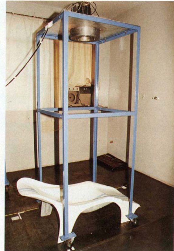
32. The improvised whole body counter used in Goiânia.
