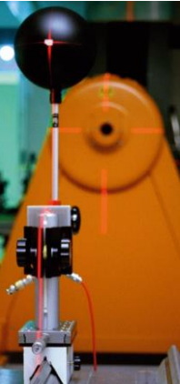
Calibration of a reference mammography ionisation chamber at the IAEA Laboratory in Seibersdorf
