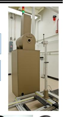
The end user of the chamber can later use the value of  $N_K$  (provided by NIST) to measure the air kerma rate,  $\dot{K}_{user}$  (in Gy/s) of a radiation field as:
