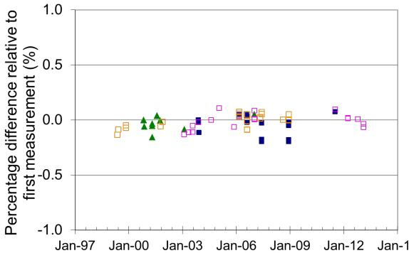
Reproducibility of the  $^{137}$ Cs irradiators is reflected in the reproducibility observed over years of the air kerma coefficient  $N_K$  of reference class chambers calibrated in these gamma-ray beams
