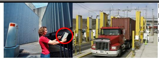
Radioactive shipments arrive at ports of entry by cargo ships, rail and trucks. Measurements are made with Radiation Detector instruments tested with <sup>137</sup>Cs
