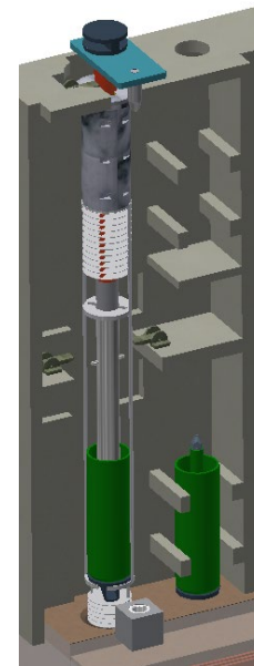
Sketch of U/TRU co-deposition module, US Patent 10,301,729
