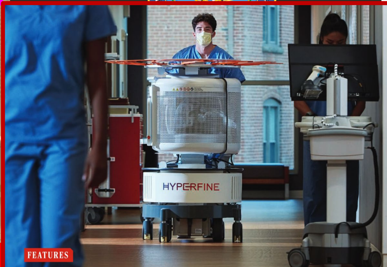
Hyperfine's Swoop, the first U.S. FDA-approved low-field brain scanner, can be wheeled to a patient's bedside.
