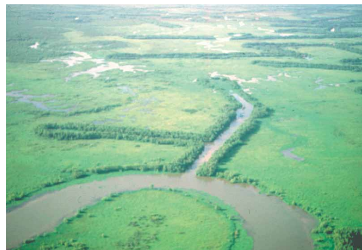
Figure 9: Canals dredged for drilling platforms and access to well heads from a natural channel. More dredged access canals can be seen in the background (Source: N.N. Rabalais, LUMCON).
