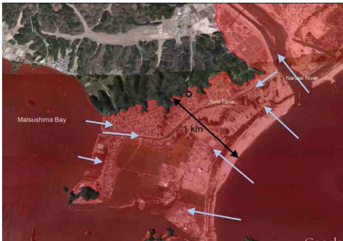
FIGURE 14 Approximate inundation area in the west area of Higashimatsushima City. This region was particularly vulnerable because the tsunami attacked from several directions. The star marks the location of the evacuation building shown in Figure 15. Note its proximity to higher ground on the hillside. Source: EERI, 2011
