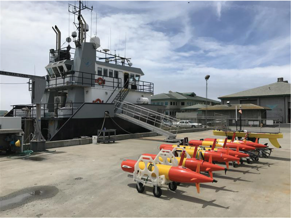
FIGURE 6 A fleet of long range AUVs (Hobson et al., 2012) fitted with different imaging, water sampling, and eDNA collection payloads alongside a Liquid Robotics Wave Glider, all readied for deployment in Monterey Bay. The fleet of vehicles is able to coordinate observations for an extended period of time to provide a multifaceted view of dynamic ecosystem processes (after Zhang et al., 2021a, b). Susan von Thun © 2017 MBARI.
