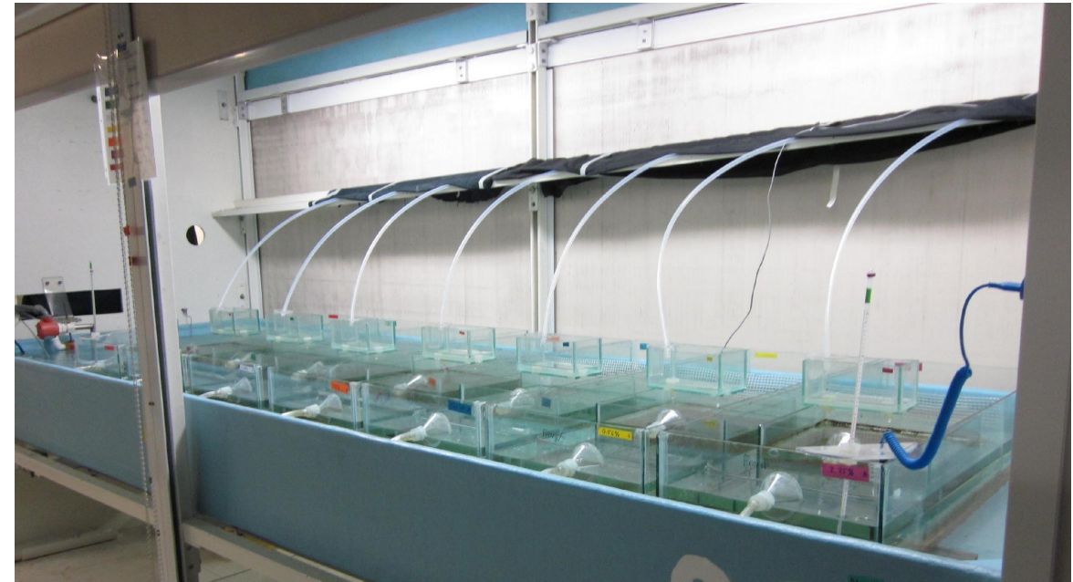
Single replicate table of large-scale fish exposures at the EPA Gulf Breeze Laboratory. Each tank housed fish exposed to a unique concentration.
