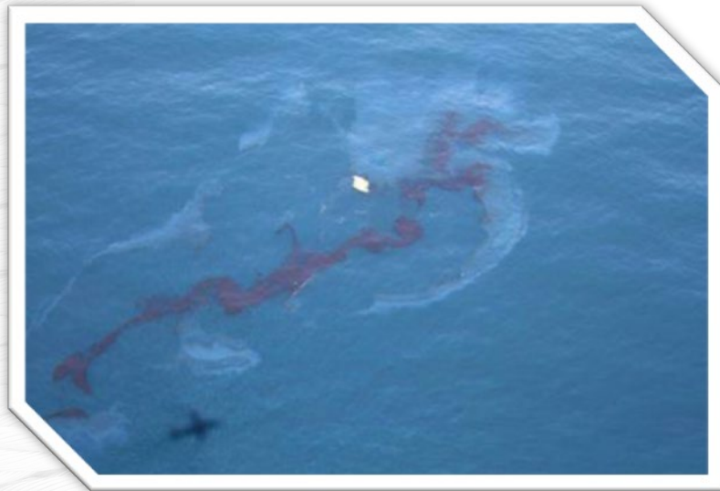
Test slick after herder application, pre-burn
