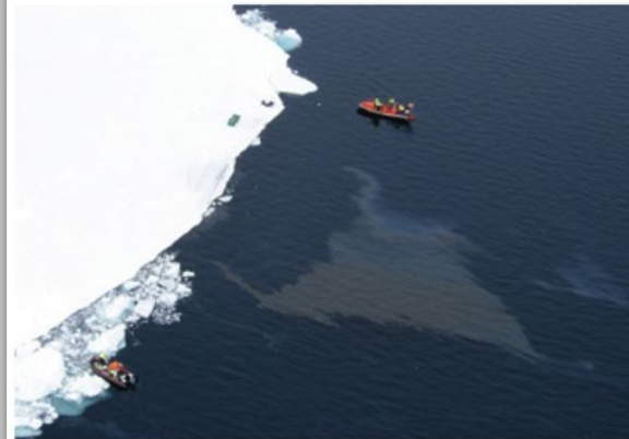
Herders enabled in situ burning during a 2016 field test offshore Norway. Left photo shows herded slick and right photo show unherded slick.
