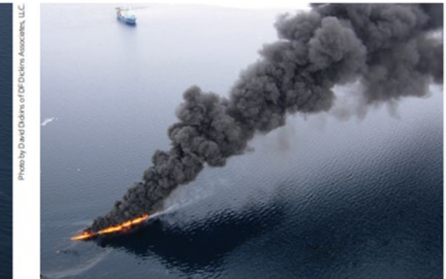
Herders enabled in situ burning during a 2016 field test offshore Norway. Left photo shows herded slick and right photo show unherded slick.
