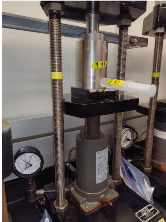
Pore water extraction via squeezing on the JOIDES Resolution
