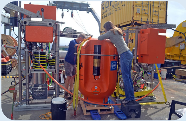
One-of-a-kind RCA Cabled Shallow Profiler Moorings
