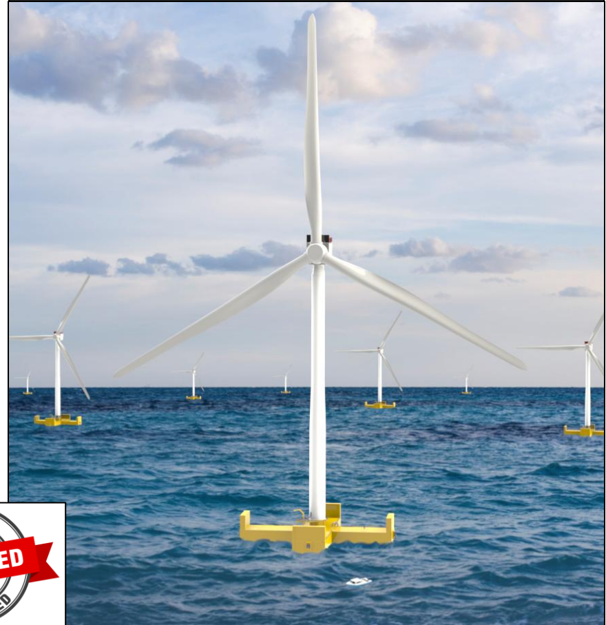
VoltturnUS+ cruciform barge with passive damper 1:4 Scale deployment (2025) Nylon semi-taut mooring
