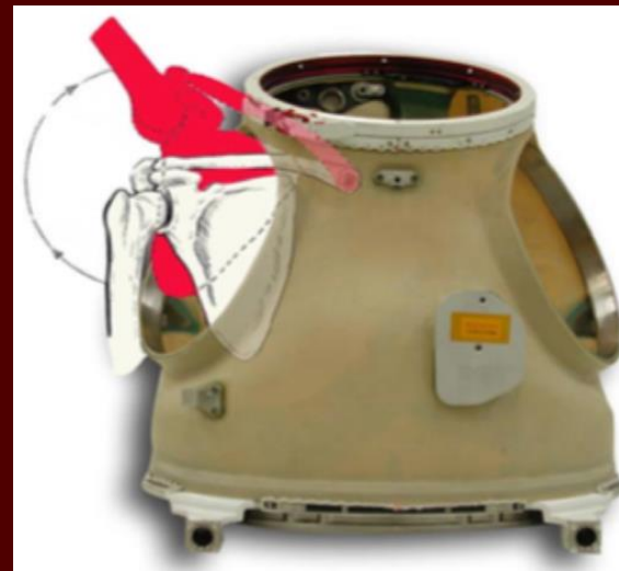
Restricted shoulder motion by hard upper torso (HUT) assembly
