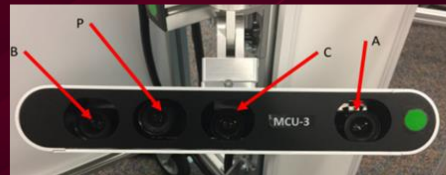
3dMD Motion Capture MCU Consisting of Two Black and White Cameras (A & B), One Color Camera (C), and a Speckle Pattern Projector (P).
