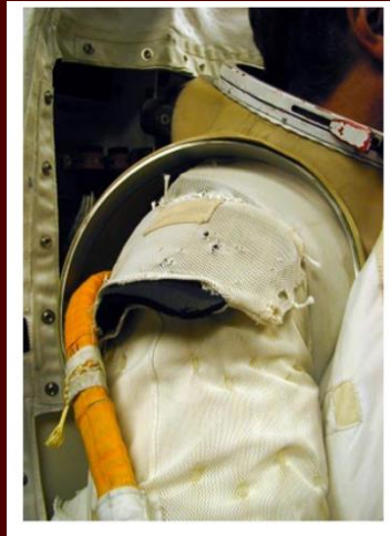
Shoulder clearance between scye bearing and liquid cooling and ventilation garment.
