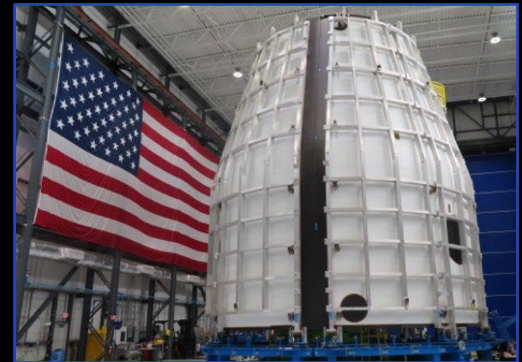
Universal stage adapter structural qualification article panels aligned and loaded on Vertical Assembly Tool
