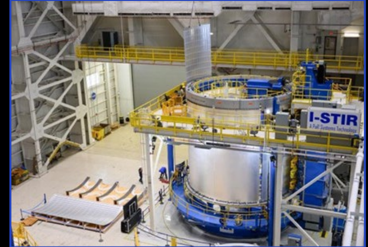
Liquid hydrogen tank for core stage in progress
