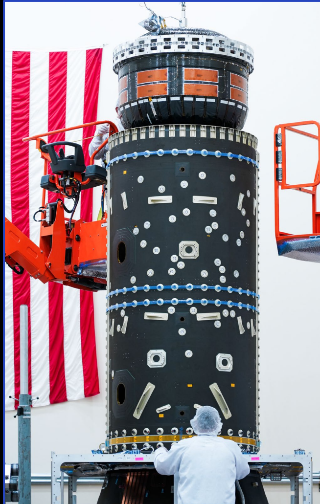
Maxar technicians installed xenon tanks into Power and Propulsion Element (PPE) central cylinder for Gateway
