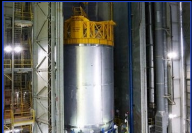
Core stage liquid oxygen tank at Vertical Assembly Center at Michoud
