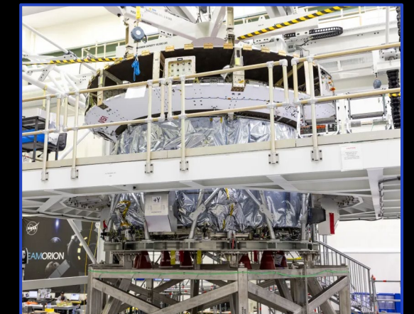
European Service Module 3 joined with Crew Module Adapter
