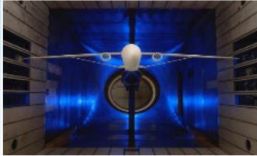
Transonic Truss-Braced Wing 5-10% fuel burn benefit
