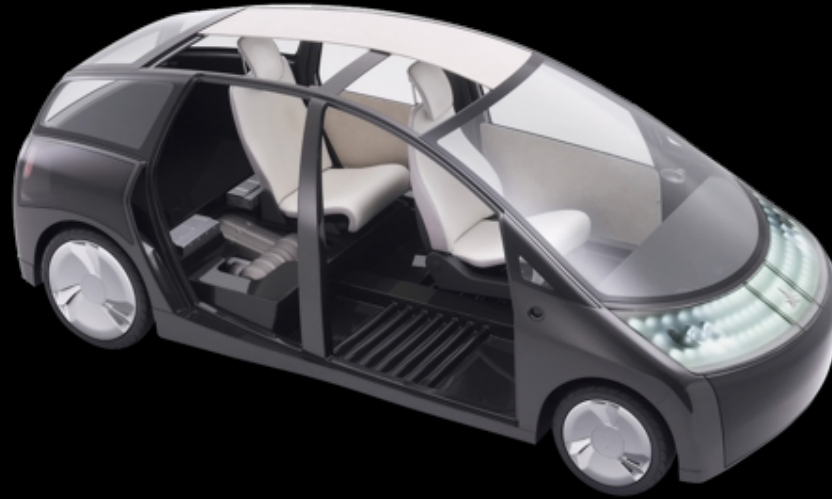
Toyota 1/X carbon-fiber plug-in hybrid concept sedan (2007) Prius size, 1/2 fuel use, 1/3 weight (420 kg, or 400 kg as a non-plug-in hybrid—70% lighter)
