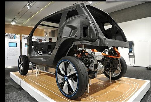
BMW i3 2013's ~120–150-kg carbon-fiber-composite passenger cell, m 0 1,250 kg
