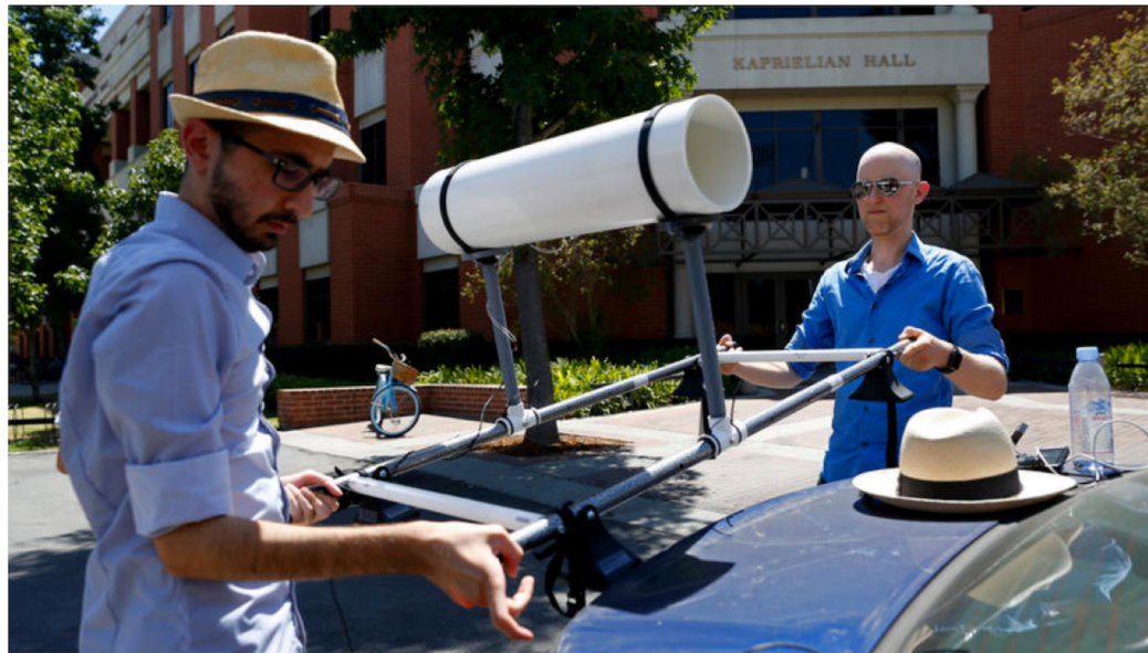
George Ban-Weiss, right, with environmental engineering graduate student Arash Mohegh, removes a mobile thermometer sensor from the roof of the car the team drives through Los Angeles neighborhoods searching for pockets of heat. (Gary Coronado / Los Angeles Times)
