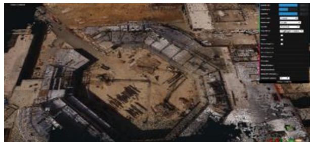
Virtual Comparison: 4D As-built Model (Progress) vs 4D BIM (Plan)
