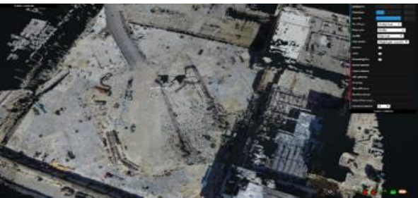
Virtual Comparison: 4D As-built Model (Progress) vs 4D BIM (Plan)
