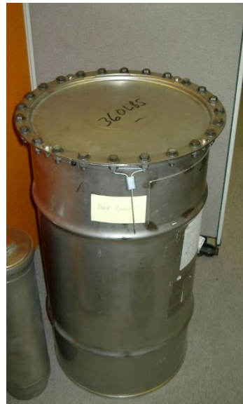
Type B - 9975 Plutonium Shipping container (~400 pounds)
