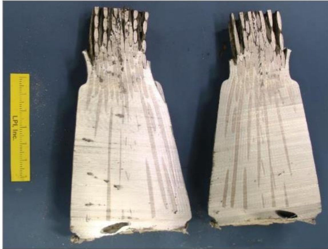
Zinc casting was cut open and macroetched to reveal zinc grain and/or flow structure.
