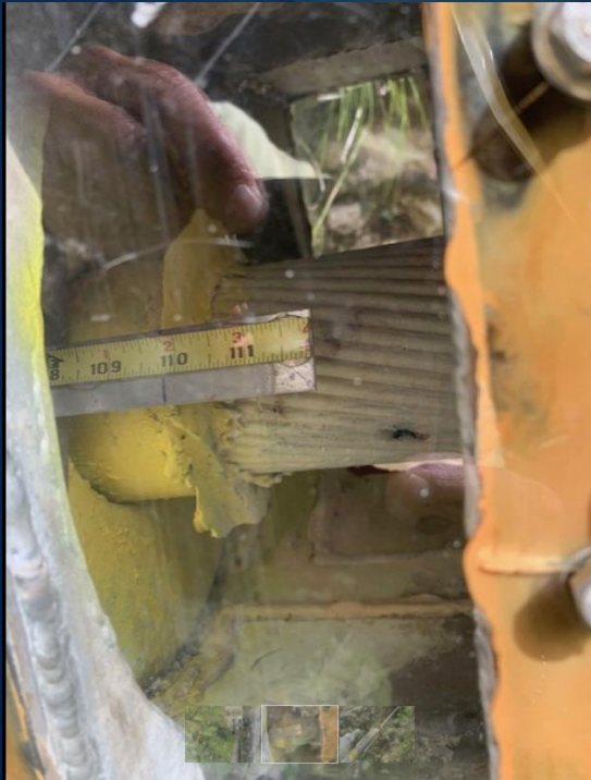
Image: Tower 12 auxiliary backstay socket separation
