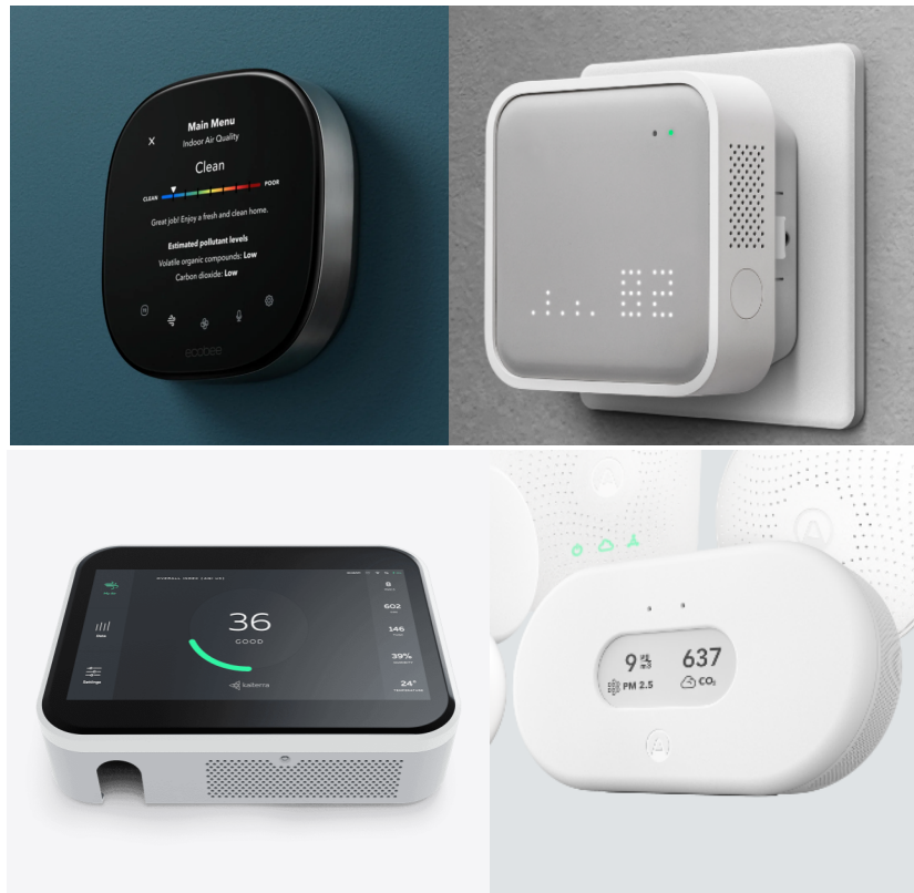
fig. 5.12 Examples of Integrated IAQ Sensors on the Market (clockwise from top left: Ecobee Thermostat Premium; Awair Omni; Airthings Space Pro; Kaiterra Sensedge).
