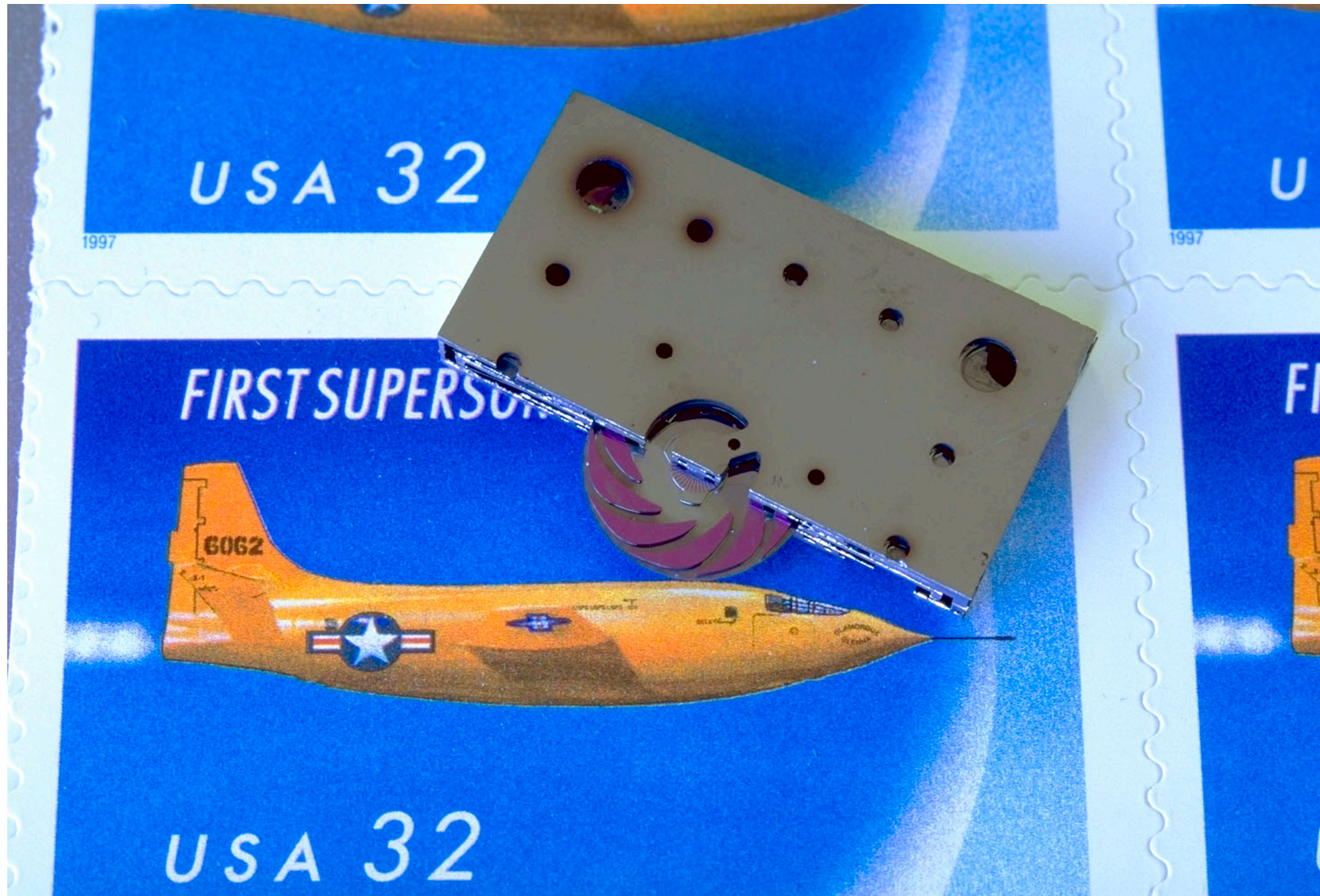
50W Microengine in a BA-5590 package
