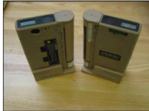
25W Reformed Fuel Cell 24% eff on Methanol
