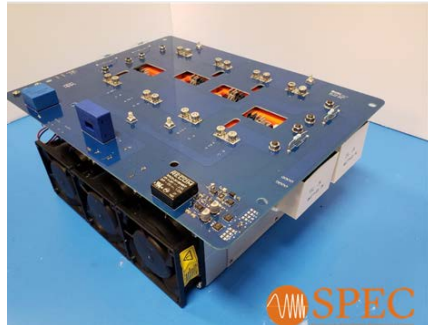
Fig. 1: A tested module near the required performance level. Improved thermal management may make 30 kW/kg possible.
