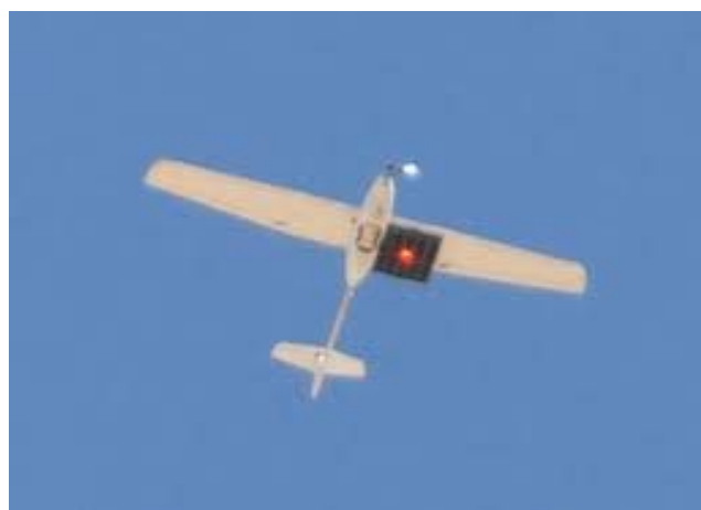
LaserMotive outdoor laser power to UAV (2012)
