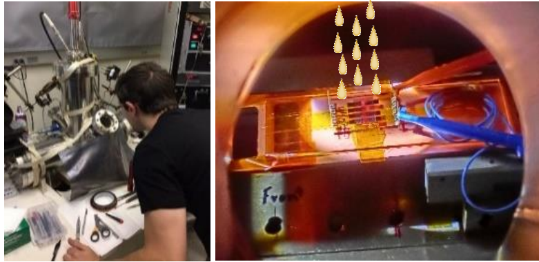
Figure 1. EC devices exposed to electron beam in vacuum chamber simulating isotope stimulation.
