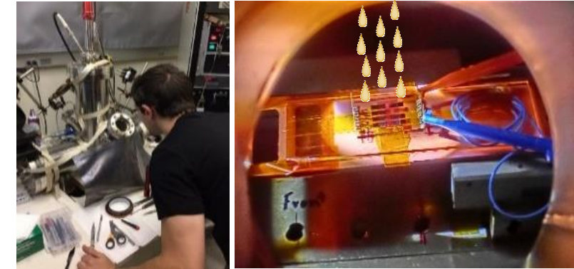
Figure 1. EC devices exposed to electron beam in vacuum chamber simulating isotope stimulation.
