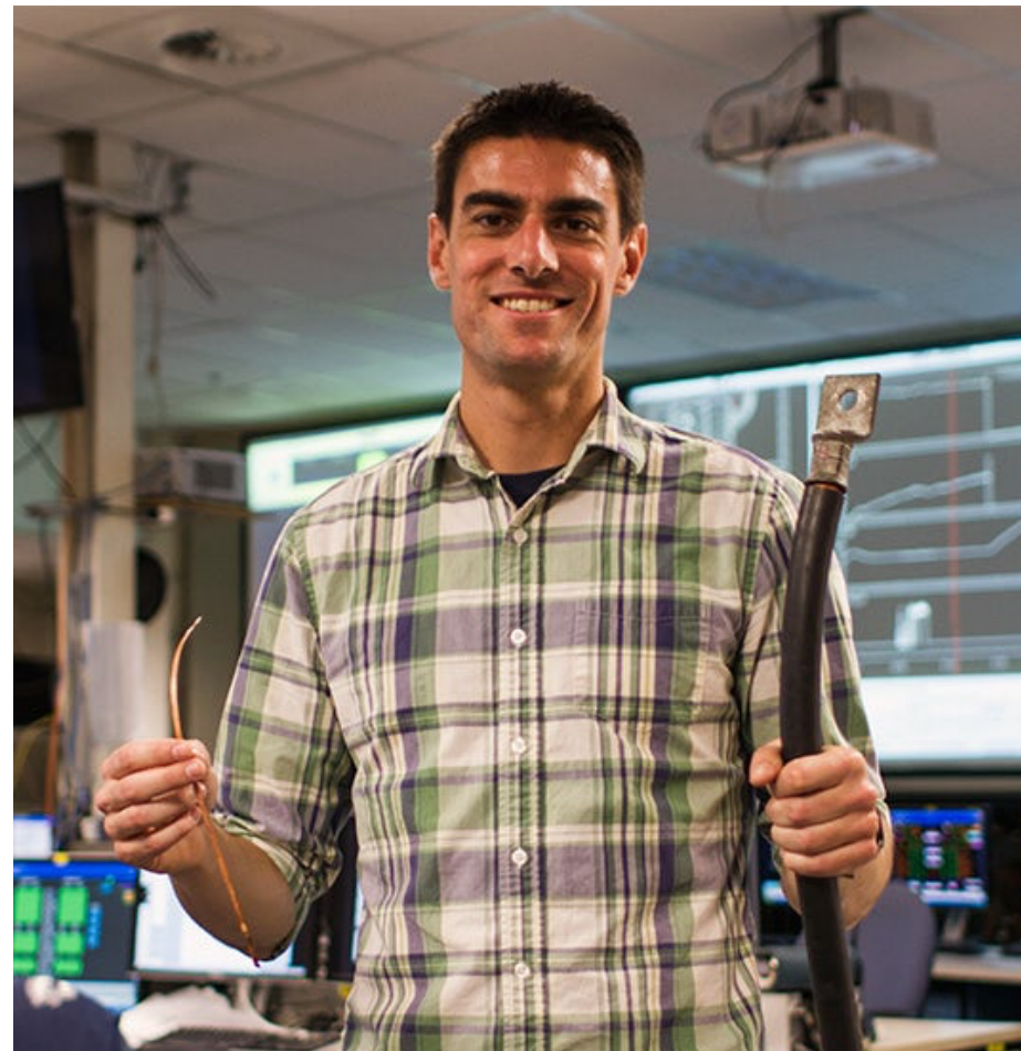
Brandon Sorbom (CFS) compares REBCO superconducting tape to copper buss
