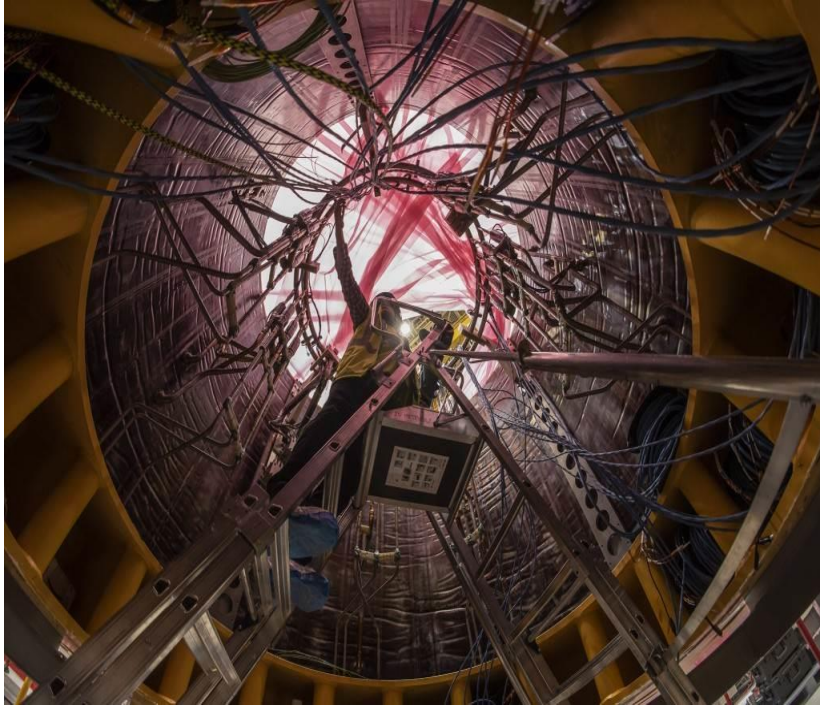
A look inside the first central solenoid module. Five more will stack on top to complete the 18-meter-tall system
