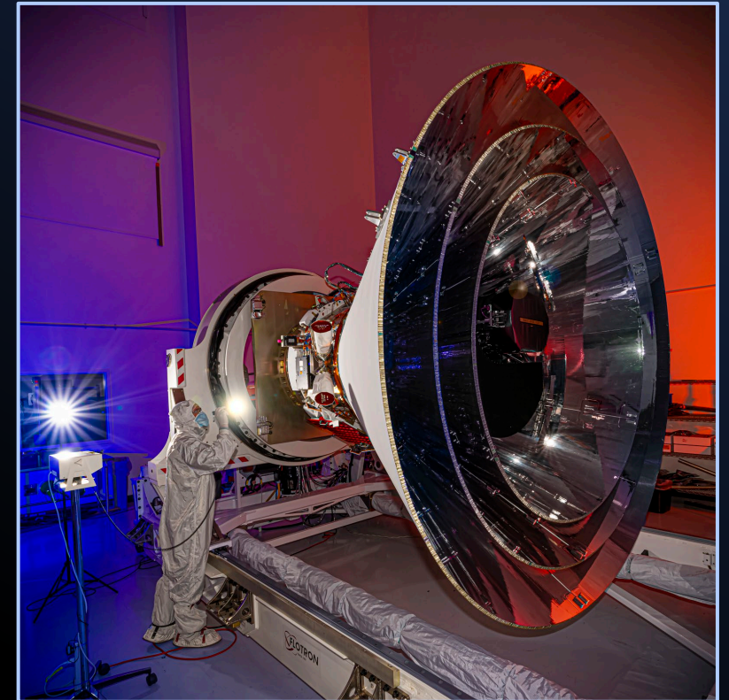
SPHEREx observatory in a horizontal position, showing all three layers of photon shields as well as the telescope. Credit: BAE Systems, Courtesy NASA/JPL-Caltech.
