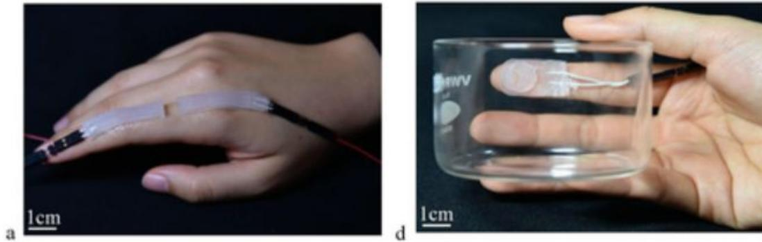
Demonstration of the functionalities of the strain and force sensors as wearable devices for human motion detection
