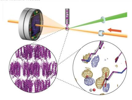
Diffract before destroy – SFX + optical pump laser
