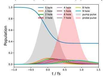
Collisional electron impact dominates valence ionization after initial photoionization. (1000 water molecules in box,  $\lambda_{mfp} \sim 1$  nm,  $E_{kin} \sim 220$  eV)
