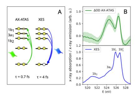
AX-ATAS @ 0.7 fs shows no evidence for two structural motifs in ambient liquid water
