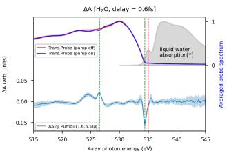
Signature of valence holes and pre-edge bleach Scan pump  $\omega$  and probe  $2\omega$  over O K-edge ~600 as pump & probe pulses @ 600 as delay 0.2 eV spectrometer resolution Pump-off w/ Ar gas attenuator
