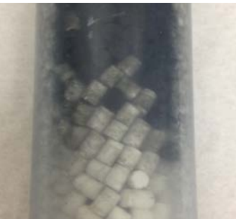
Sabatier catalyst material after vibration testing
