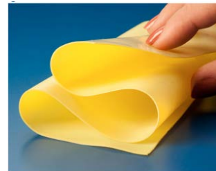
Mechanically Robust Polymer Aerogels Demonstrated as Substrates for Conformal Antennas
